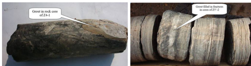
Fig. 4.33 Core samples at select grout holes
